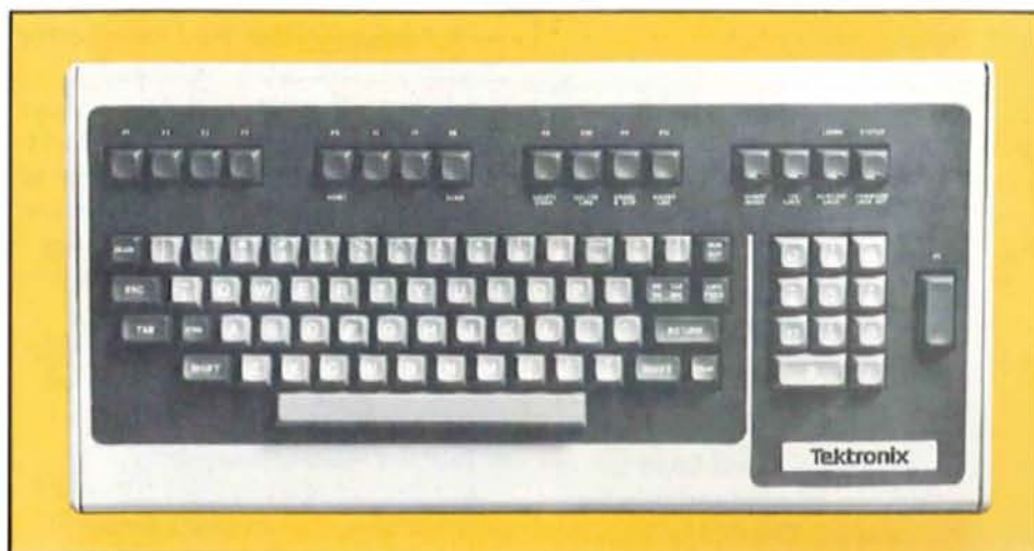
Fig. 2. The keyboard features a standard office typewriter layout plus a numeric pad and sixteen user-definable keys. In the LEARN mode, virtually every key can be programmed for another character or character string.
