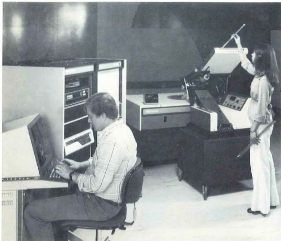
Fig. 1. Tek uses its own S-3200 Series Test Systems to perform incoming inspection on millions of parts annually.
