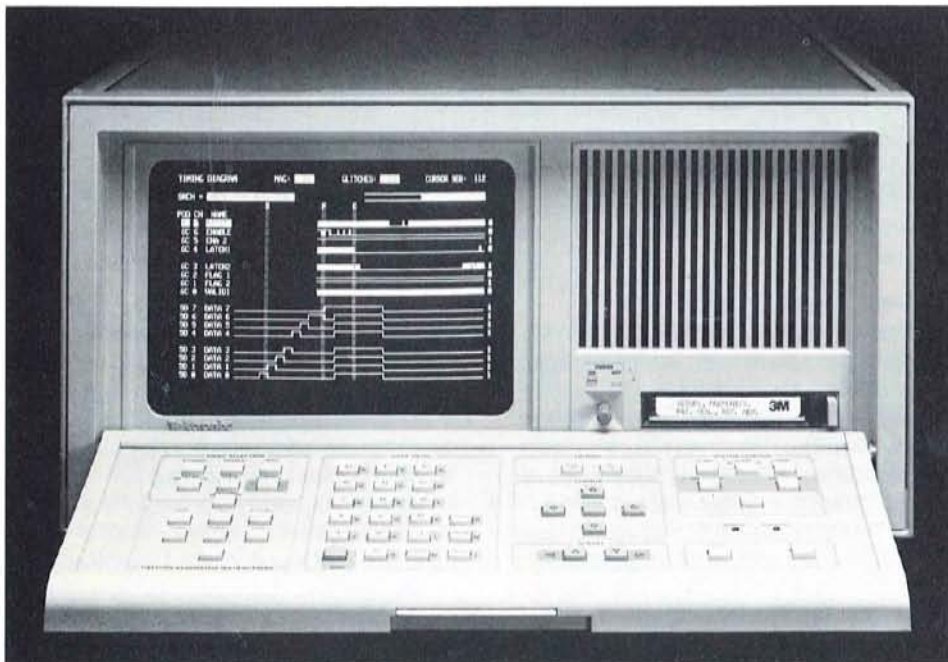
Fig. 1. The DAS 9100 Digital Analysis System provides a choice of performance via plug-in card modules. An easy-to-use keyboard, selectable menus, and a large, bright display facilitates operation.
