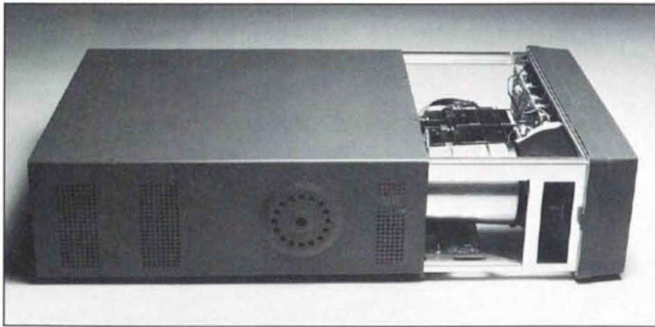
Figure 4. The one-piece cabinet provides structural strength, helping to eliminate the need for heavy structural members.
