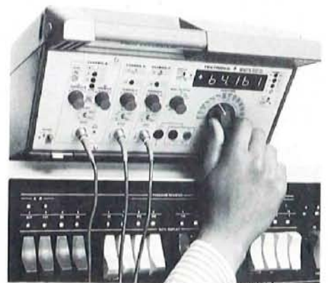
Fig. 1 The sloping front panel of the 851 provides good visibility and easy access to controls whether the unit is sitting on the floor, the workbench, or atop a computer cabinet as in this photo.
