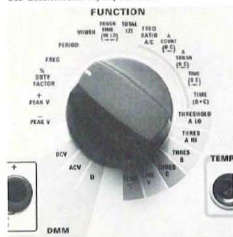
Fig. 2 The function switch allows the operator to select which one of twenty-two functions will be performed and arranges the internal circuitry to accomplish it.
