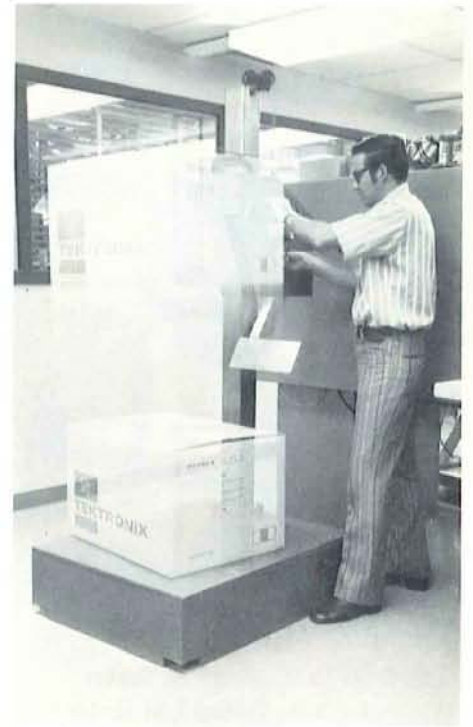
Fig. 6. A unit undergoes drop test to ensure packaging will prevent damage to instrument during transit.
