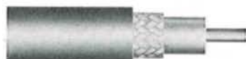
Flat Ribbons Instead of Round Wires for Shield Reduce Losses Above About 1 GHz
