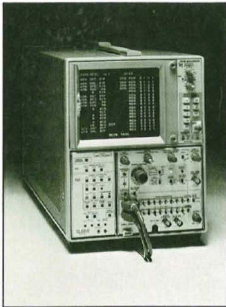
Fig. 3. The 7D01 Logic Analyzer with the DF2 Display Formatter converts any 7000-Series Mainframe to a Logic Analyzer with seven ways to look at logic.
