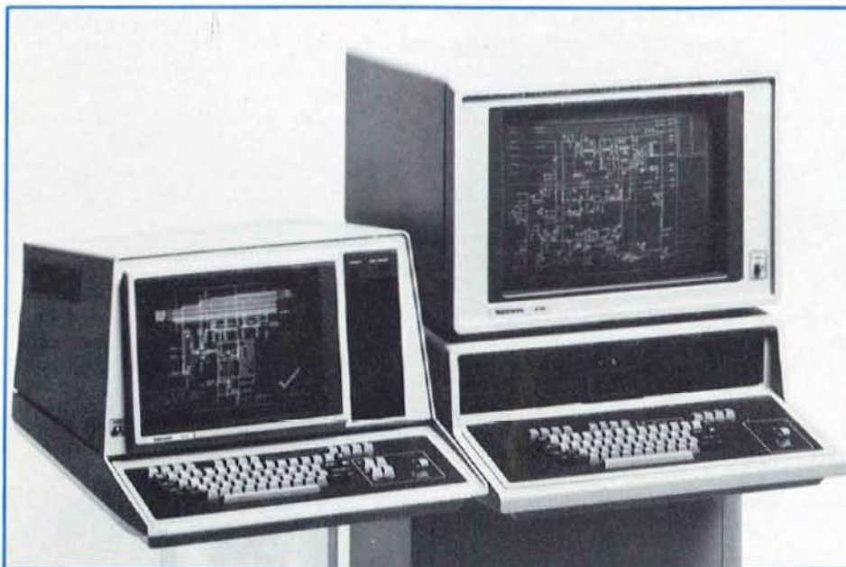
Fig. 1. The new 4112 raster-scan terminal (left) and the 4114 DVST terminal (right) provide users a choice of graphics display capability with features designed to greatly increase the user's productivity. The 4112 and 4114 are software compatible with the 4010 Series terminals.
