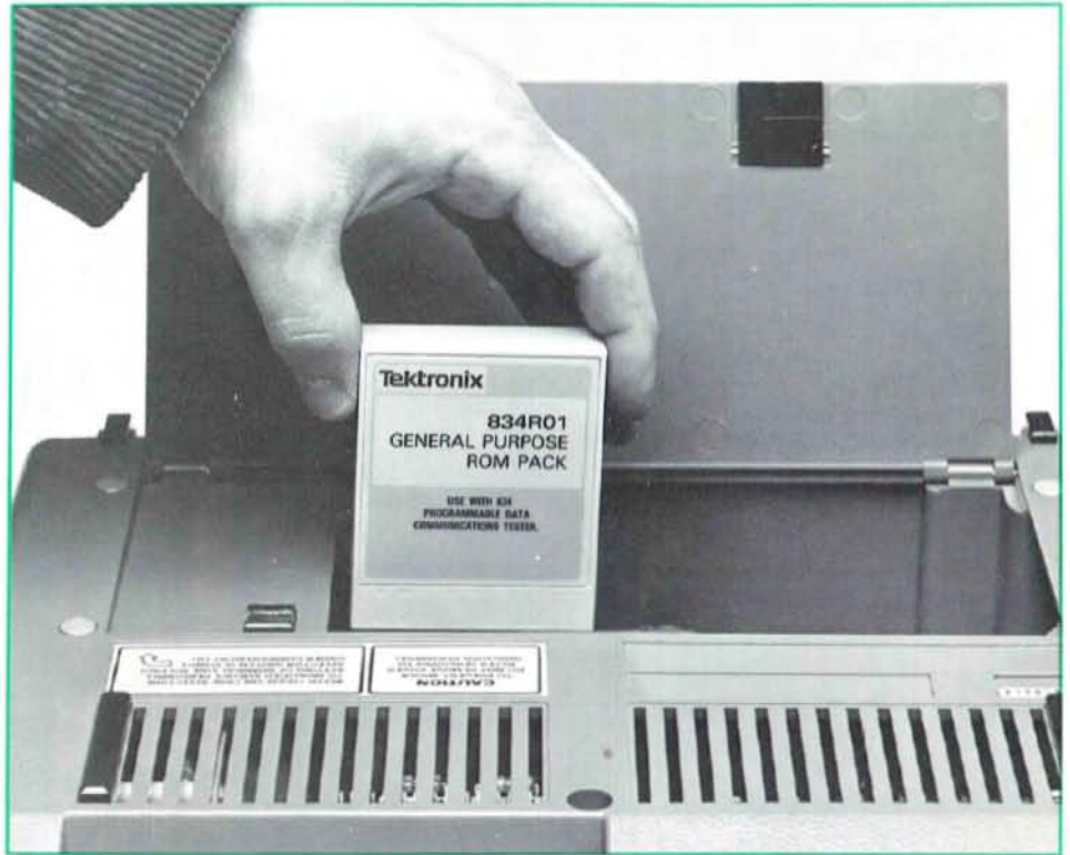
Fig. 2. Through the use of ROM Packs, the user can expand the capability of the 834 and employ programs customized for the system under test.
