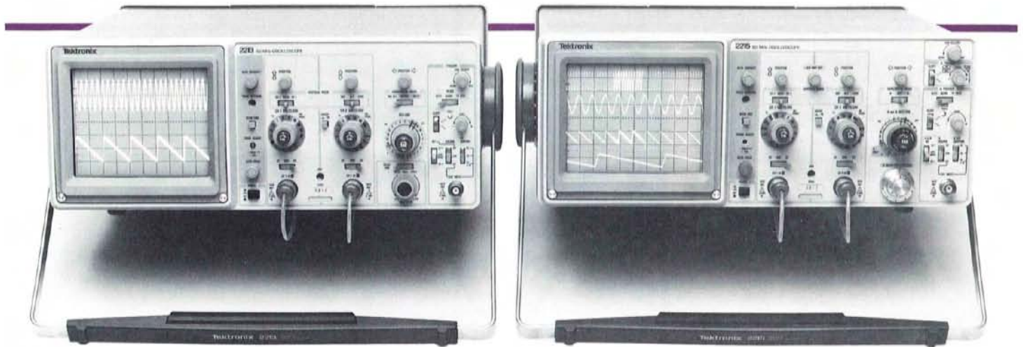
Figure 1. The Tektronix 2213 and 2215 Portable Oscilloscopes provide 60-MHz dual-trace, delayed-sweep operation and a full 8 by 10 cm display in a package weighing only 13.5 pounds (6.1 kg).
