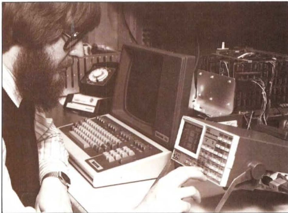
Fig. 2. Versatility, operating ease, and small size make the 308 useful in a wide range of applications. Here the 308 is being used to analyze graphic terminal operation.
