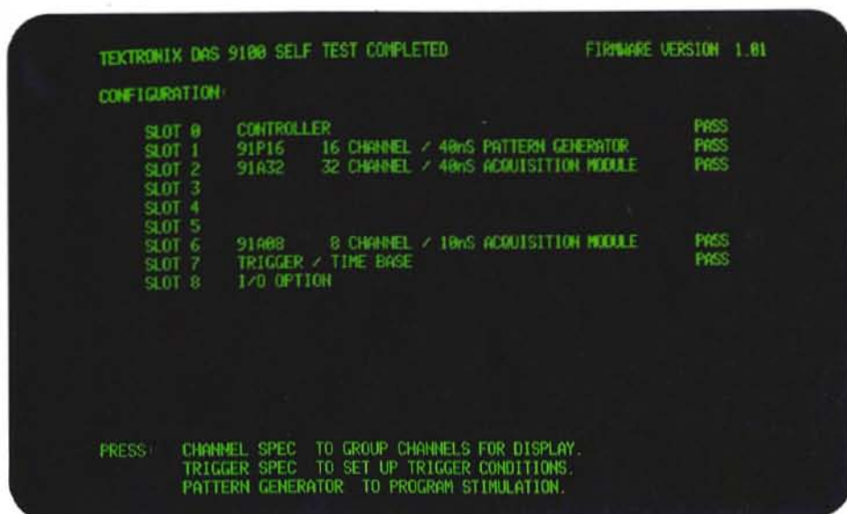
Fig. 12. The Configuration menu is automatically displayed at power-up. It lists the installed modules, the firmware version resident in the DAS, and whether each module passes or fails the power-up self-tests.
