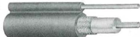
Steel Messenger Wire Supports Flexible Cable When Suspended Between Poles
