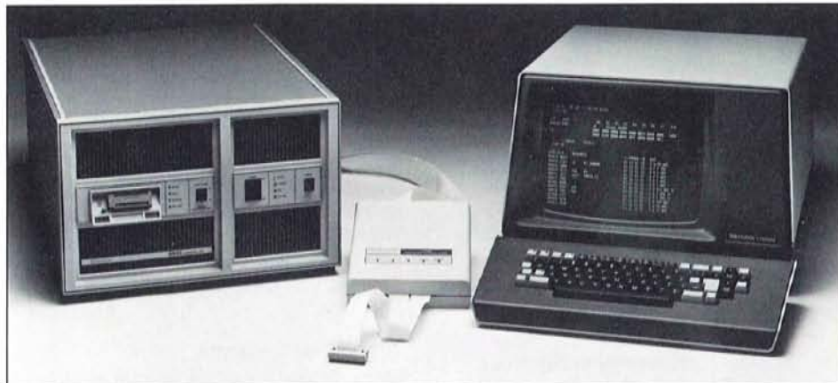
Figure 1. The 8540 Integration Unit, pictured with the CT8500 CRT Terminal and prototype control probe, provides complete coverage of the hardware/software integration process during microcomputer design.
