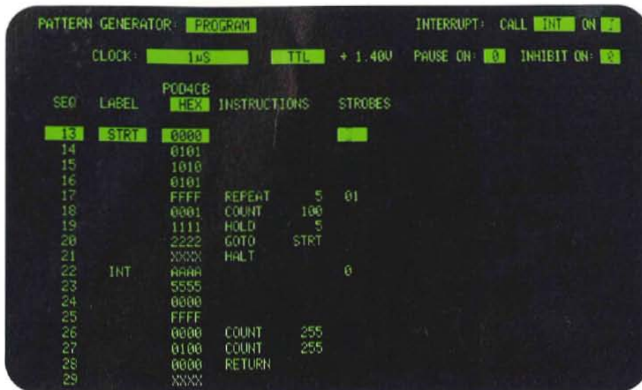
Fig. 9. The Pattern Generator Program sub-menu is used to set up the pattern generator's output program and select the programmed strobes.
